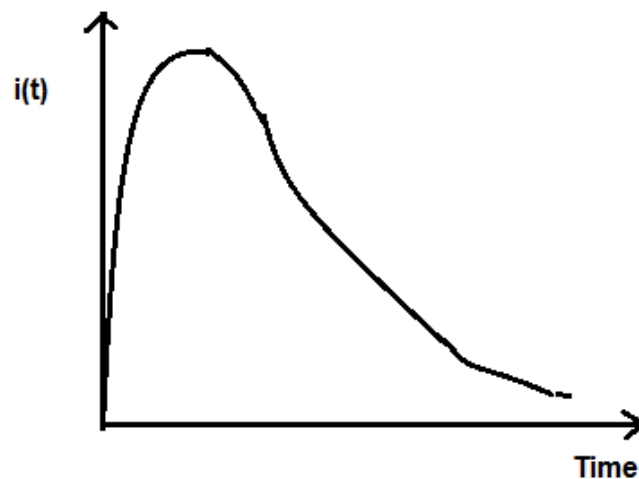
Fig 2.7 Current response in over damped case
