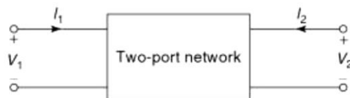
Figure: 6.1 Two-port network
